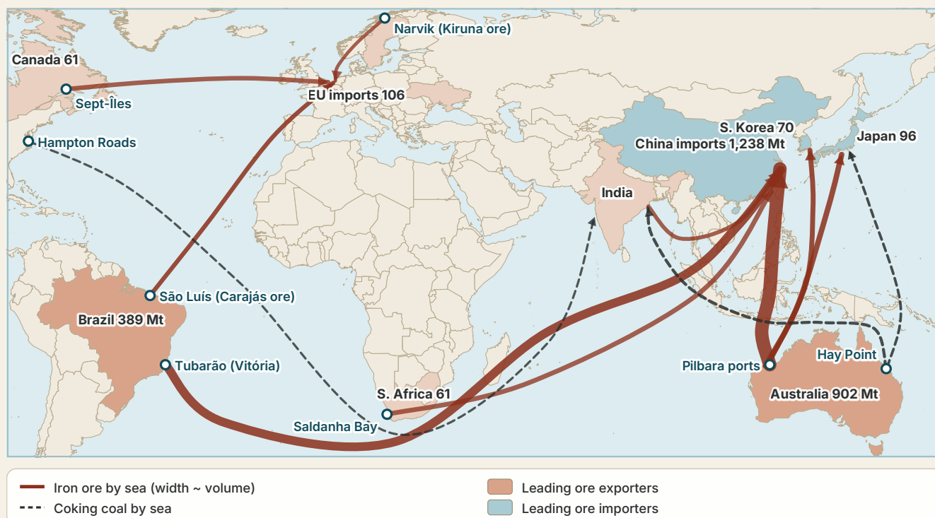
Fig. 11.20 Main iron ore flows (arrow width roughly proportional to volume, 2024) and coking coal routes. Exporter and importer totals in million tonnes. Source: worldsteel, World Steel in Figures 2026; routes generalised.
