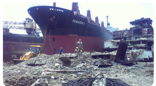
Fig. 19.7 A tanker beached for dismantling at Alang on the Gulf of Khambhat; its steel will be re-rolled in Gujarat's mills.
