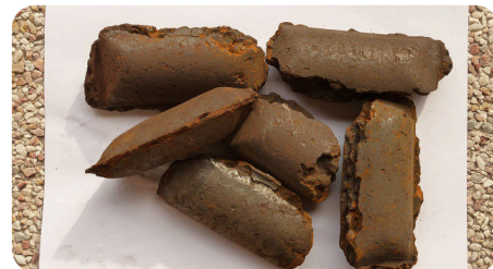
Fig. 11.4 Hot briquetted iron, sponge iron pressed into dense pillow shapes so it can be shipped.
