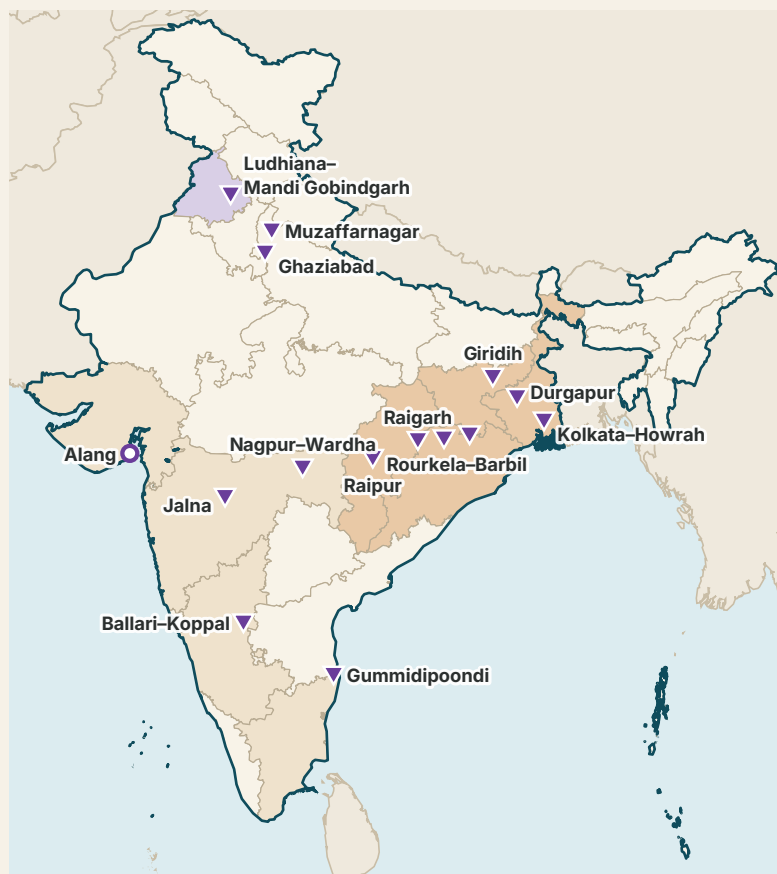
Fig. 11.10 Main clusters of sponge-iron, induction-furnace and re-rolling units. The eastern states host kiln-based sponge iron near ore and coal; Punjab, western Uttar Pradesh, Maharashtra and Tamil Nadu melt scrap near markets; Alang supplies ship-breaking scrap.
